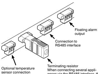
When connecting several appliances via the RS485 interface, the terminating resistor must remain on the last appliance. Remove the terminating resistors from the appliances in between.
